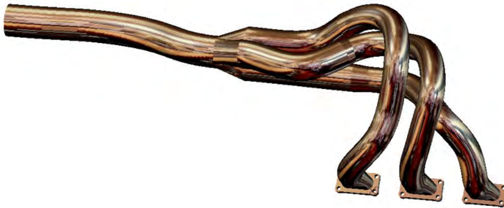
Figure 8: CAD image of W-9 exhaust system.
