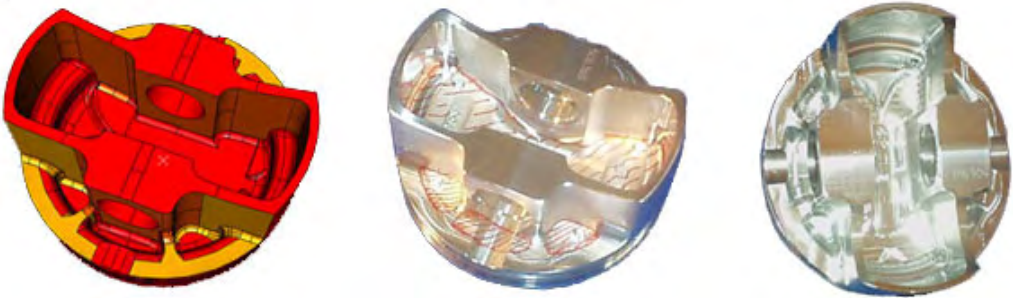
Figure 20: CAD image of the W-9 piston, unmodified piston, and machined piston.
