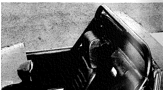
Roll bar cage is anchored to the frame that forms part of the floor pan. Windows were cut into the boxed member to fit in gusset plates for reinforcement.
